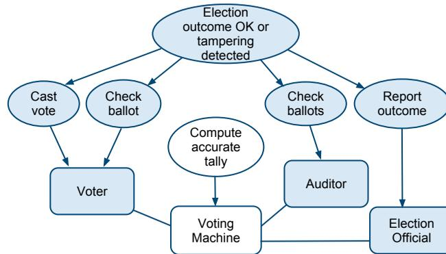
Fig. 4. Property-part diagram for an end-to-end voting system.
