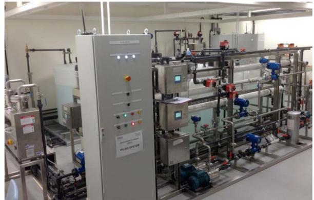
**Figure 1:** Secure Water Treatment (SWaT) testbed
