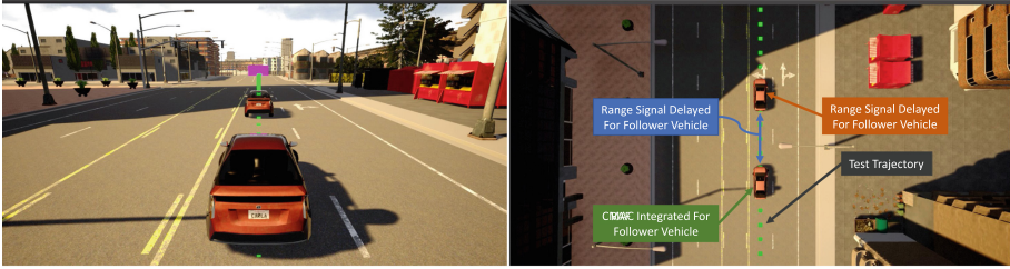
Fig. 2. Test scenario for evaluation of the ACC case study
